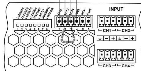
\*Short the two VC inputs to control all channels
